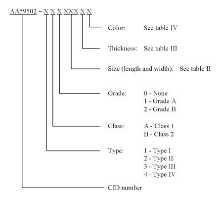
EXAMPLE: AA59502-3A1084J1 would be Type III, Class 1, Grade A, sheet which is 8 feet long by 4 feet wide, 0.1 inch thick, and with natural color.
